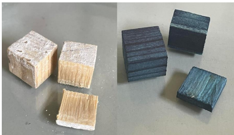
Fig. 1. Photos of impregnated pine wood cubes, under same impregnation condition, with (left) Zn 2 /Al 1 -CO 3 layered double hydroxide and (right) Indigo Carmine.
