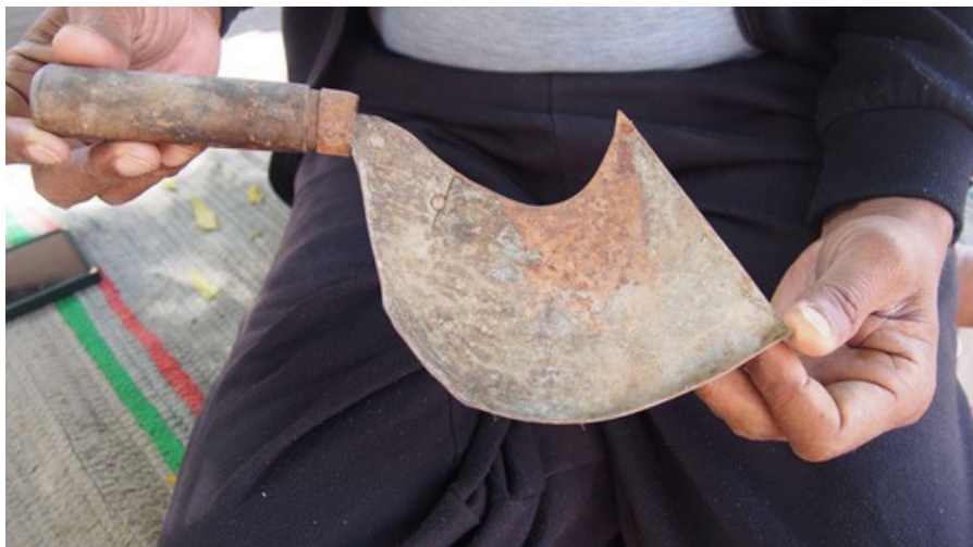
Fig. 5. Charpala – a traditional tool used for collecting leaked opium latex from a cut poppy shell (17 February 2022, Daru, Madhya Pradesh; photograph by the author).
